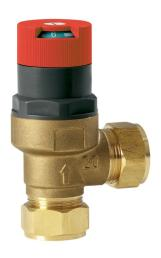
Regulates heating system differential pressure High capacity flow up to 50 litres per minute Differential pressure range 0.1 to 0.6 bar 22mm compression fitting
