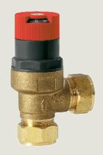
The Tower ABBV1 should be fitted where a boiler bypass is required. Typically this is the case when a system is equipped with thermostatic radiator valves (TRV's), and to allow pump overrun operation after zone valves have closed down.
